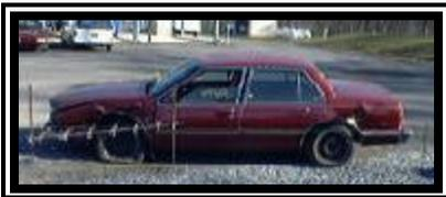
**Figure 4. Left side surface damage to the 1988 Oldsmobile Delta 88 Royale.**
