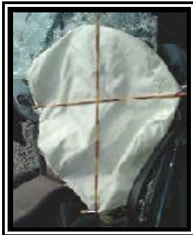
Figure 7. 1998 Honda Civic EX redesigned passenger air bag.
