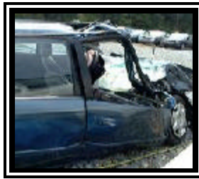
Figure 4. Underride damage to the greenhouse area.
