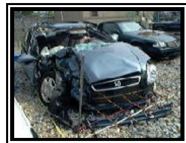
Figure 2. Frontal damage to the 1998 Honda civic EX.
