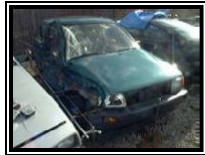
Figure 4. Right side surface damage to the 1993 Ford Festiva.
