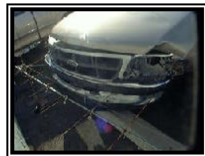
Figure 3. Frontal damage to the 1998 Ford F-150 pickup truck.
