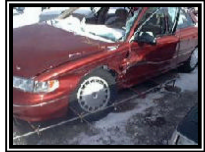
Figure 4. Left front side surface damage to the 1998 Buick Century Custom.
