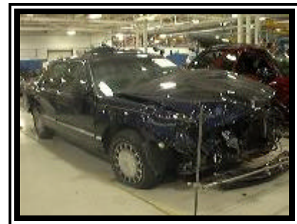
Figure 3. Frontal damage to the 1998 Cadillac Deville.
