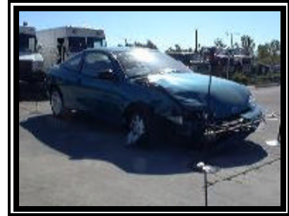
Figure 3. Front right damage to the 1998 Chevrolet Cavalier.
