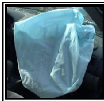
Figure 6. 1999 Toyota Corolla redesigned passenger air bag.
