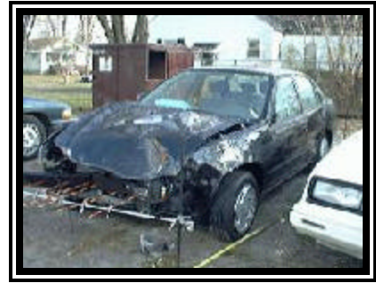
Figure 3. Frontal damage to the 1999 Toyota Corolla.
