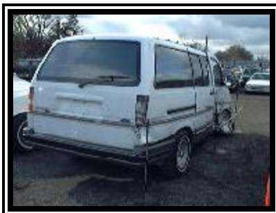
Figure 4. Right side surface damage to the 1991 Ford Aerostar.
