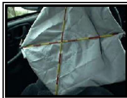
Figure 6. 1998 Chevrolet S-10 redesigned driver air bag.
