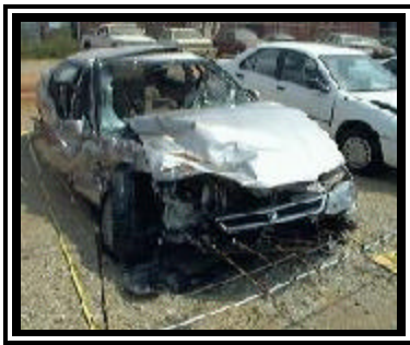
Figure 4. Frontal damage to the 1996 Honda Accord EX.
