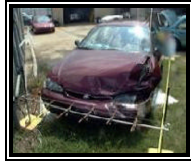
Figure 3. Frontal damage to the 1998 Toyota Corolla.
