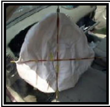
Figure 6. 1998 Toyota Corolla redesigned driver air bag.
