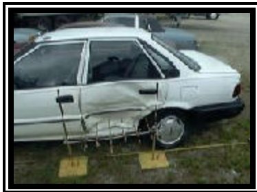
Figure 4. Left side surface damage to the 1992 Geo Prizm.
