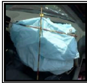
Figure 7. 1998 Toyota Corolla redesigned passenger air bag.
