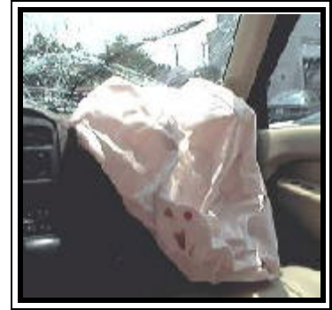
Figure 6. 1998 Nissan Pathfinder redesigned passenger air bag.
