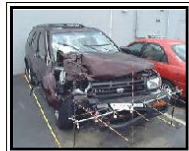
Figure 3. Frontal damage to the 1998 Nissan Pathfinder.
