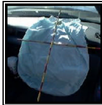
Figure 7. 1998 Nissan Sentra redesigned passenger air bag.
