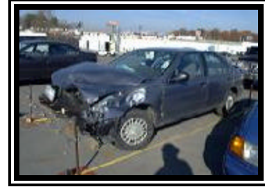
Figure 3. Frontal damage to the 1998 Nissan Sentra XE.
