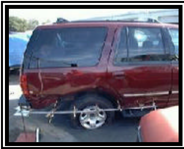
Figure 4. Right rear side surface damage to the 1998 Ford Expedition.
