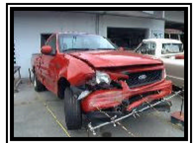
Figure 2. Frontal damage to the 1998 Ford F-150 pickup truck.
