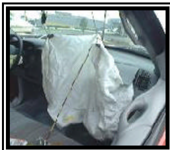
Figure 5. 1998 Ford F-150 redesigned passenger air bag.
