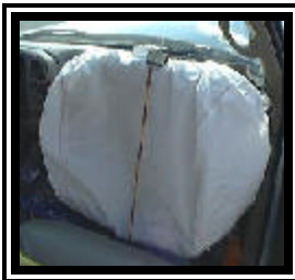
Figure 6. 1999 Chevrolet Tahoe redesigned passenger air bag.
