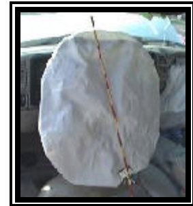
Figure 5. 1999 Chevrolet Tahoe redesigned driver air bag.
