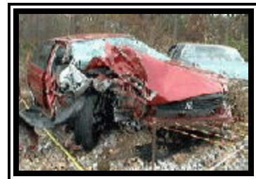
Figure 2. Frontal damage to the 1998 Honda Civic LX.
