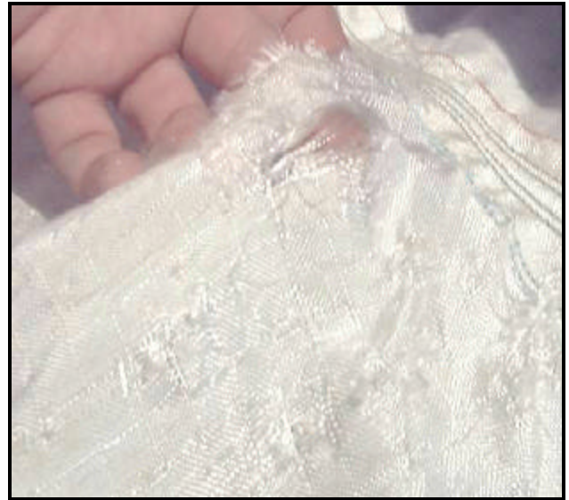
Figure 6. Interior, case vehicle. Passenger's side air bag damage (holes & fraying).
