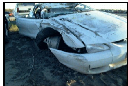
Figure 3. Exterior Vehicle 1 showing initial front, right impact damage
