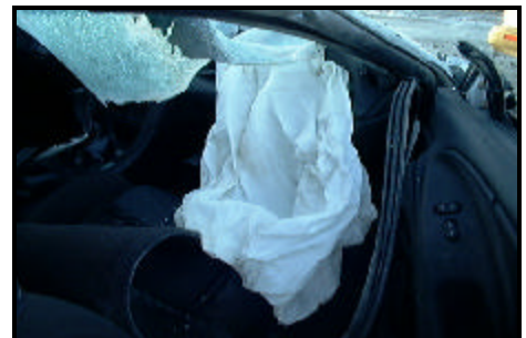
Figure 10. View showing deployed passenger (front, right) air bag
