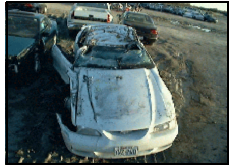
Figure 4. Overhead view showing rollover damage to Vehicle 1.
