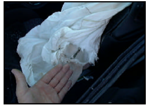
Figure 8. View showing hole in passenger air bag
