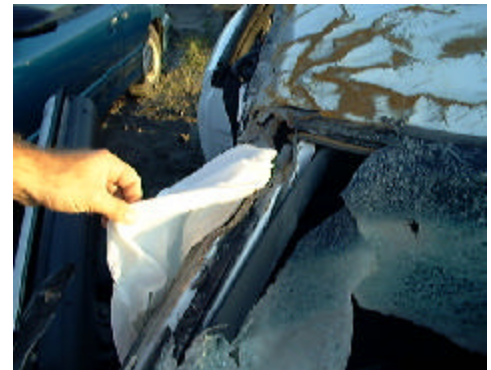
Figure 9. Passenger air bag melted to the right A-Pillar
