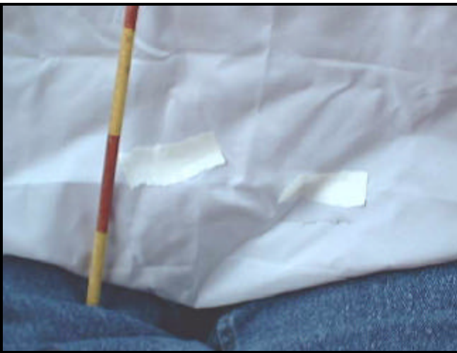
Figure 7. Interior, case vehicle. Air bag contact.
