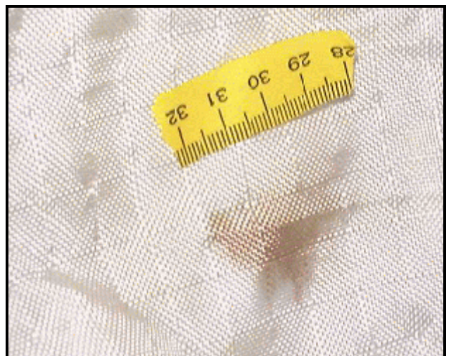
Figure 8. Interior, case vehicle. Passenger's side air bag contact evidence.
