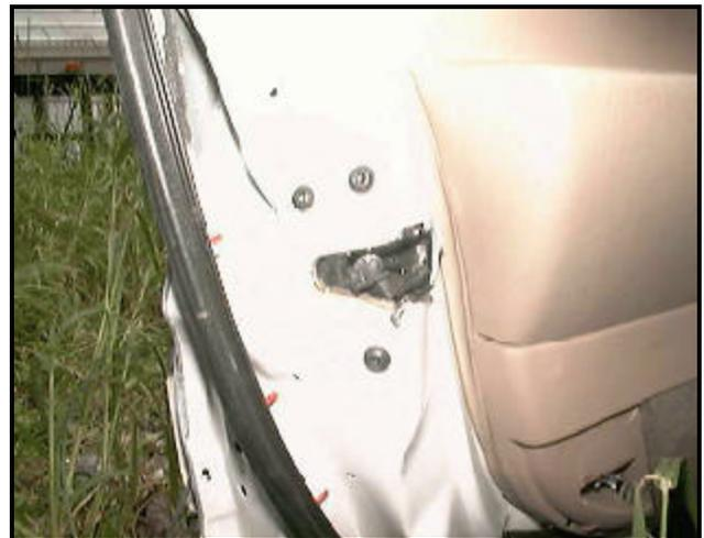
**Figure 9.** Latch/striker failure, left front door.
