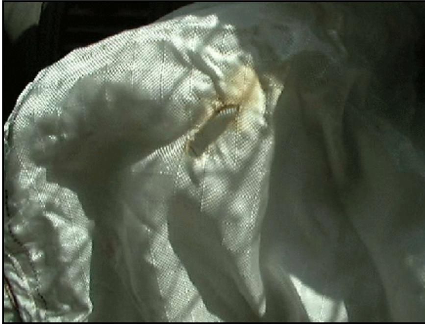
**Figure 8.** Interior, case vehicle. Passenger's side air bag (burn hole).
