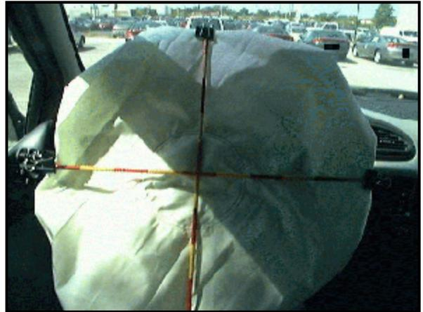
**Figure 6.** Interior, case vehicle. Driver side air bag.
