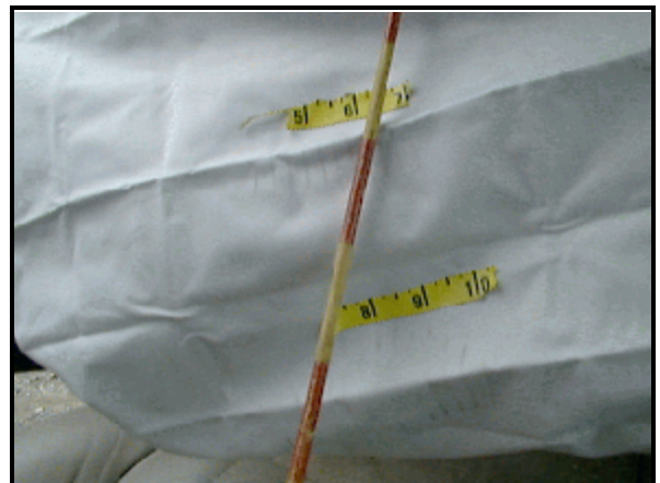
Figure 6. Close up of smudge on face of driver's side air bag
