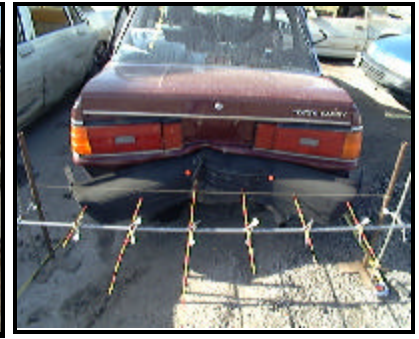
Figure 6. Impact Damage to Rear Plane of Vehicle 2
