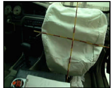
Figure 14. View showing deployed passenger (front, right) air bag
