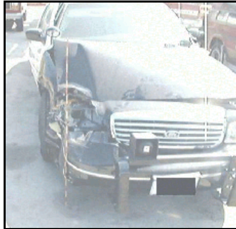
Figure 3. Direct damage, Vehicle 1 (1998 Ford Crown Victoria)
