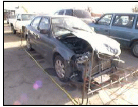
Figure 6. Three-quarter view of frontal damage
