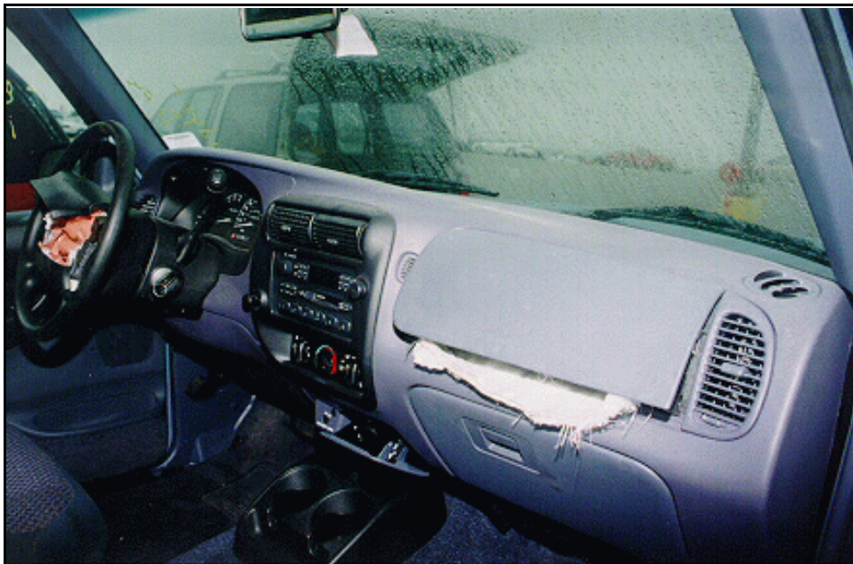
Figure 6: Case vehicle's front right cover flap; note: air bag removed (case photo #16)
