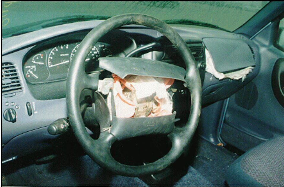
Figure 5: Case vehicle's steering wheel and cover flaps; note: driver air bag removed (case photo #13)
