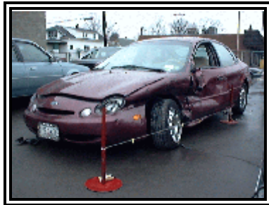
Figure 1. Left side damage to the Ford Taurus.
