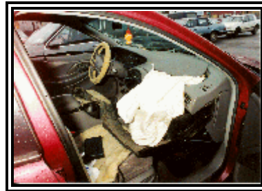
Figure 2. View of the non-deployed front left air bag and deployed front right air bag
