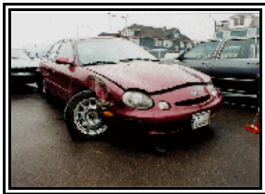
Figure 3. Right front damage to the Ford Taurus
