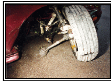
Figure 4. Separation of right front ball joint from the spindle and the fractured rod shaft
