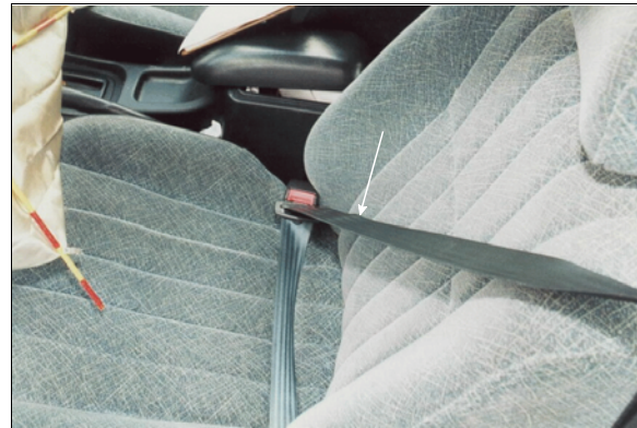
Figure 17: Case vehicle's driver safety belt showing recent (i.e., arrow points to crease in webbing) evidence of usage but not evidence of usage in this crash (case photo #42)
