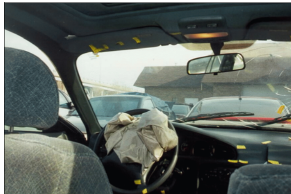
Figure 8: Case vehicle's deployed driver air bag and driver's greenhouse area showing contact to driver's sun visor and possible contact evidence on center instrument panel area (case photo #29)
