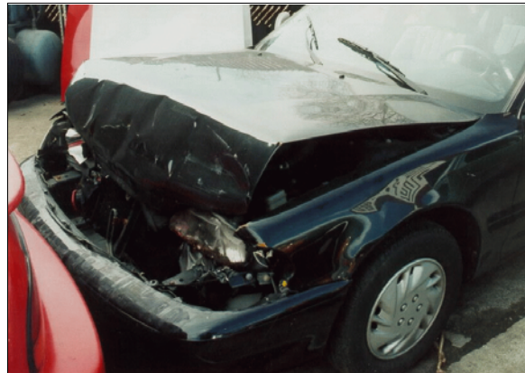
Figure 6: Case vehicle's frontal damage viewed from left of front in tow yard; Note: under-ride damage pattern and scrapes on top of front bumper (case photo #05)
