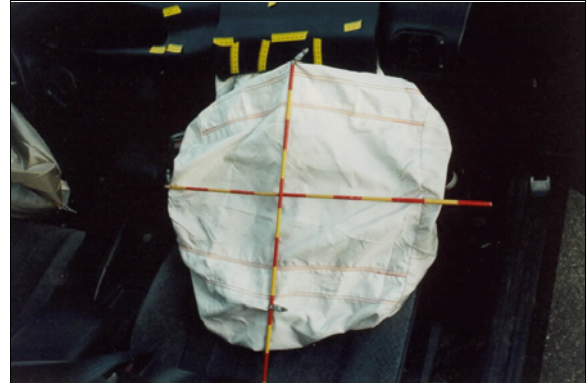
Figure 14: Front surface of case vehicle's deployed front right passenger air bag showing no obvious evidence of occupant contact and likely friction scuffs in left lower quadrant from module's cover flap (case photo #49)
