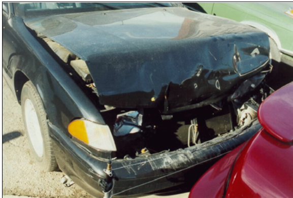
Figure 5: Case vehicle's frontal damage viewed from right of front in tow yard; Note: under-ride damage pattern and scrapes on top of front bumper (case photo #23)
