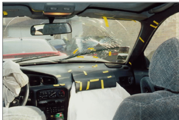
Figure 9: Case vehicle's deployed front right passenger air bag and greenhouse area showing contact evidence on front right sun visor, contacts to windshield's glazing, and possible evidence of contact to right "A"-pillar and front right air bag module's cover flap (case photo #34)
