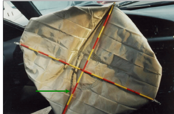
Figure 12: Case vehicle's deployed driver air bag showing makeup smear (arrow) at bottom of center circular stitching (case photo #46)
