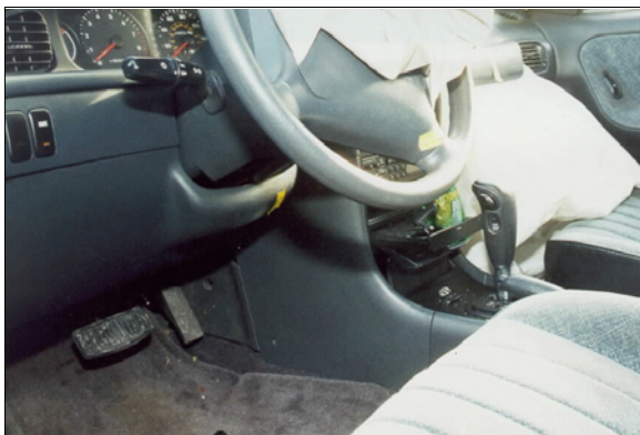
Figure 7: Case vehicle's driver seating area showing possible contact evidence on driver's knee bolster and steering wheel rim (case photo #26)
