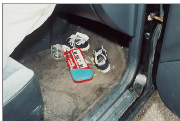
Figure 16: Floor pan area of case vehicle's front right seating position showing musical toy that most likely fractured windshield's glazing and child's shoes that were the object of conversation that precipitated the crash (case photo #45)
