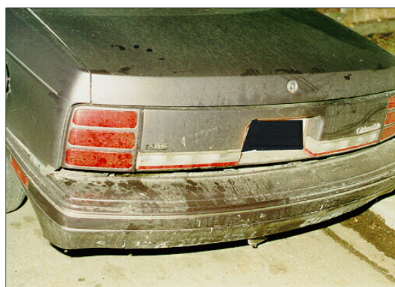
Figure 4: Damage to Oldsmobile's back bumper; Note: override damage pattern and radiator fluid stains on top surface of bumper (case photo #54)
