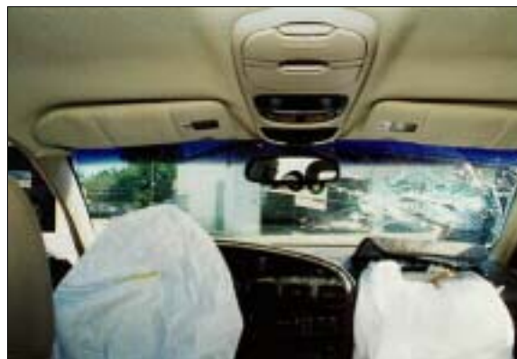
Figure 7: Case vehicle's deployed air bags; Note: make-up smear (tape) to driver air bag and deformation to front right air bag module's cover flap from striking the windshield (case photo #27)
