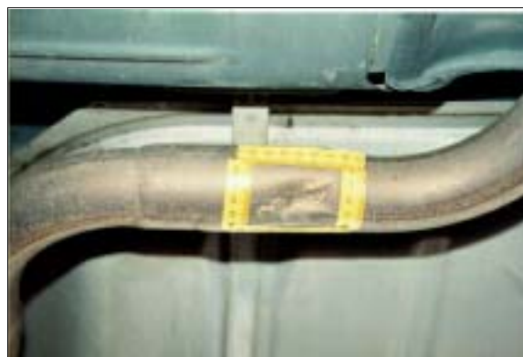
Figure 4: Close-up view of most severe dent to case vehicle's undercarriage, specifically the tail pipe (case photo #22)
