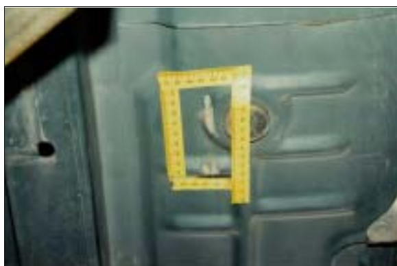
Figure 5: Contact mark to case vehicle's right undercarriage, forward of center (case photo #19)
