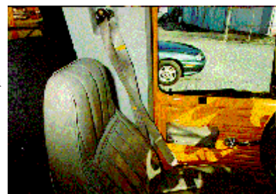
Figure 10. D-ring transfer on shoulder belt webbing.
