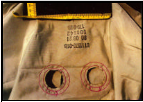
Figure 8: Close-up view of melanim transfers on the back side of the air bag.
