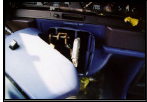
Figure 5: Fractured tilt mechanism of the steering wheel.
