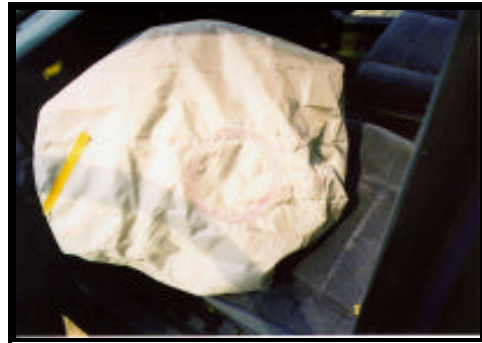
Figure 9: View of the transfer on the face of the air bag.
