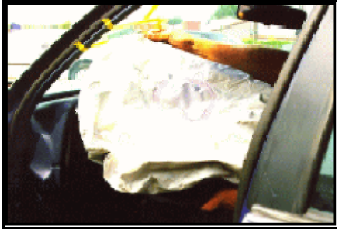
Figure 10: Altered deployment path of the air bag.
