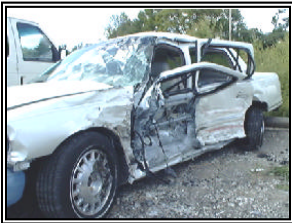
Figure 4: View of the Cadillac's left side damage.
