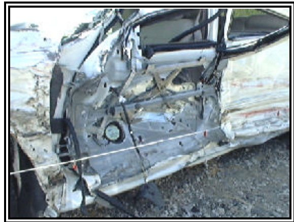
Figure 5: Close-up of the damaged left front door.
