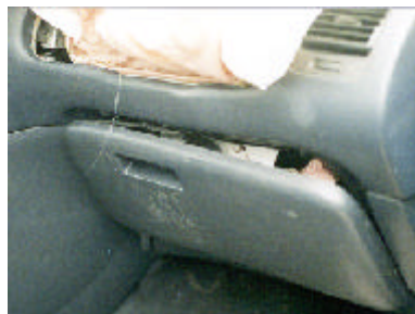
Figure 11. Passenger contact with the glove compartment door.
