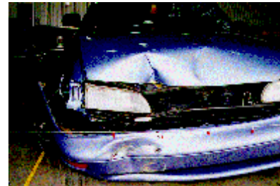
Figure 8. Close-up of damage from impacting fire hydrant.
