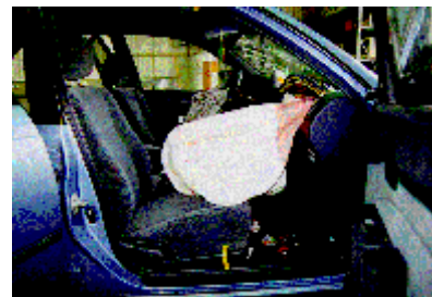
Figure 2. Profile view of front right seated position and the deployed air bag.
