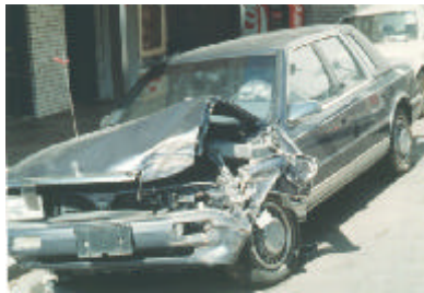
Figure 8 Corner view of the vehicle showing the area of direct contact damage at the left front corner
