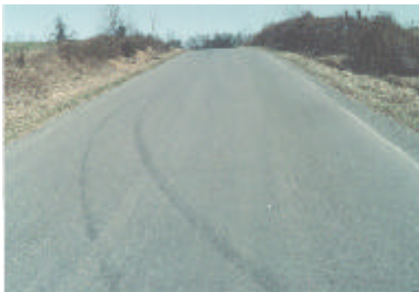
Figure 4 Reverse trajectory showing the counterclockwise scuff marks prior to the second roadway departure
