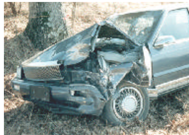
Figure 9 Lateral view of the vehicle while at the scene showing the longitudinal crush pattern and the displacement of the left front axle
