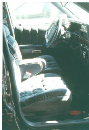
Figure 10 Lateral view of the vehicle interior taken from the right side illustrating the relative seat track positions, the steering wheel adjustment, the air bag, and the restraint belt
