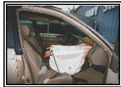
Figure 14. Excursion of the front right air bag.
