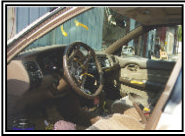
Figure 9. Driver position with air bag generant on windshield.
