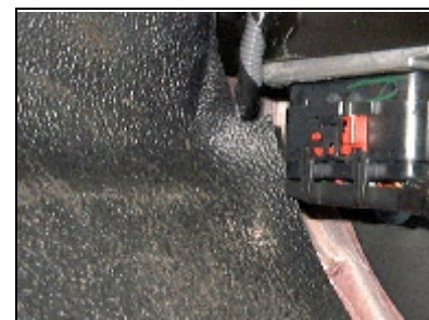
Figure 5- View of inertia shut-off switch located behind the right kick panel
