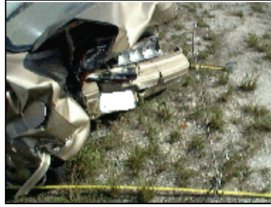
Figure 20- View showing the depth of the crush profile
