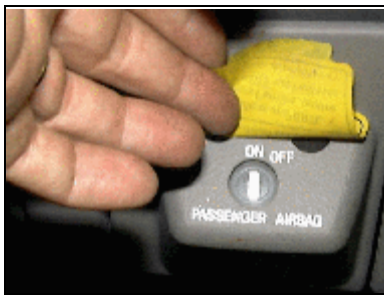
Figure 9- View of the manual shut off switch for the front right passenger air bag
