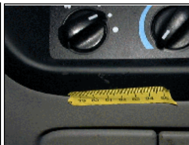
Figure 10- View of the abraded surface of the trim below the temperature control panel
