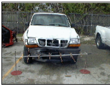
Figure 7 - View showing damage to the frontal plane of the Ford
