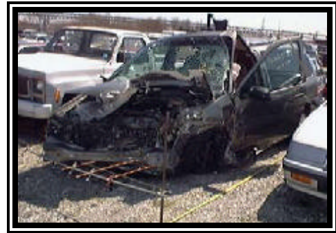
Figure 3. Front left damage to the 1998 Ford Windstar.
