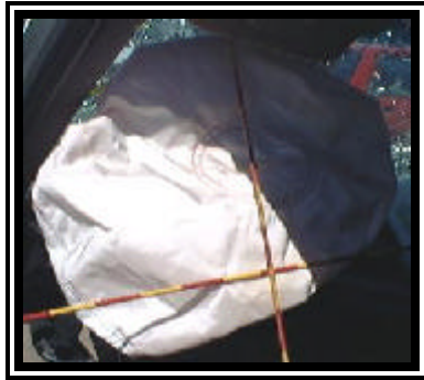
Figure 6. 1998 Ford Windstar deployed redesigned driver air bag.
