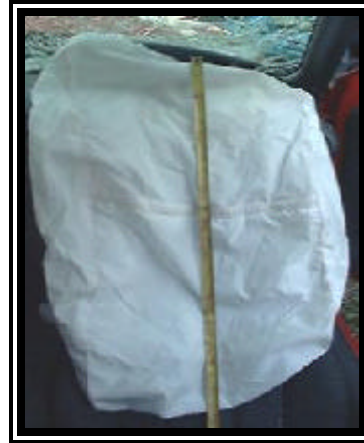
Figure 8. 1999 Pontiac Sunfire deployed redesigned passenger air bag.
