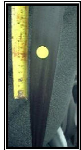
Figure 9. Loading marks to the front right shoulder belt webbing.
