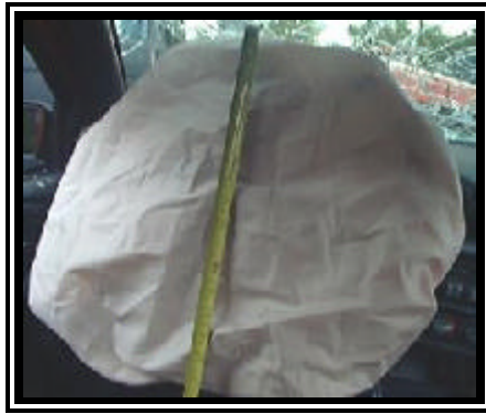
Figure 7. 1999 Pontiac Sunfire deployed redesigned driver air bag.
