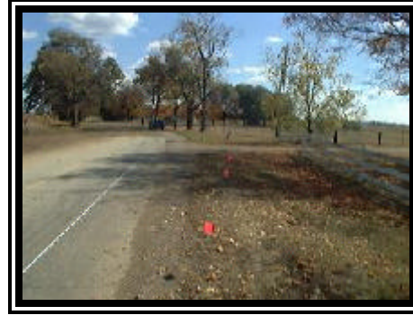
Figure 2. Pre-impact trajectory off the south pavement edge.
