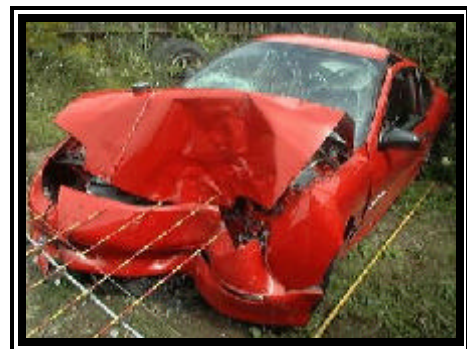
Figure 4. Front left damage to the 1999 Pontiac Sunfire.
