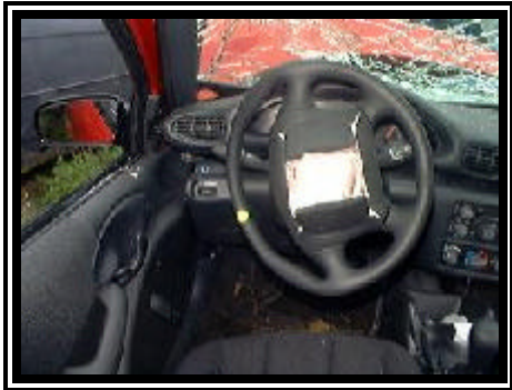
Figure 5. Deformation to the steering wheel rim.
