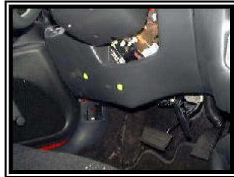
Figure 6. Scuff marks and indentations to the driver knee bolster.
