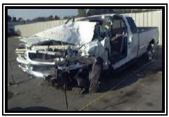
Figure 4. Front left damage to the 1998 Ford F-150 Super Cab pickup truck.
