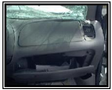
Figure 8. 1998 Ford F-150 pickup truck passenger air bag module.
