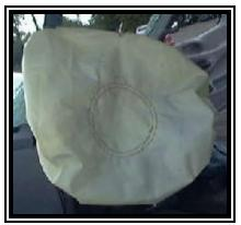
Figure 7. 1998 Ford F-150 pickup truck deployed redesigned driver air bag.
