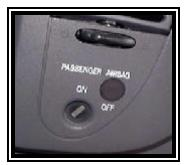
Figure 6. Passenger air bag cutoff switch (in the off position).
