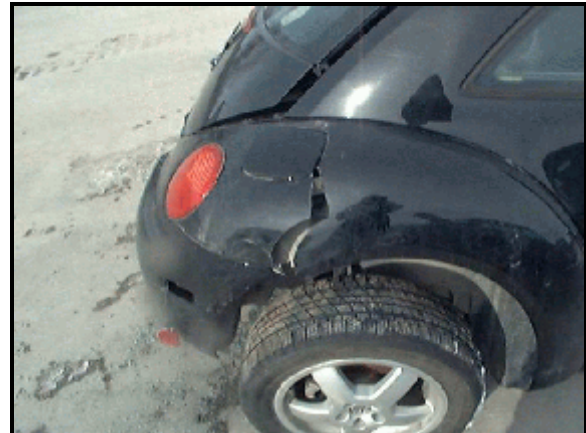
Figure 3: Minor damage on case vehicle's right rear quarter panel
