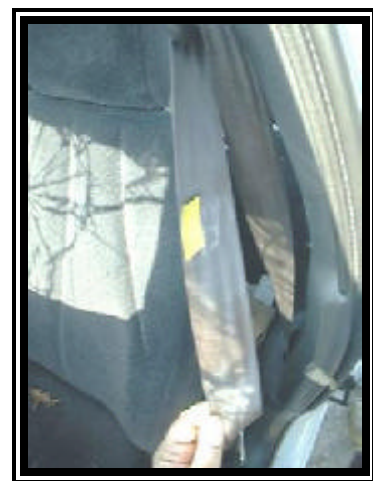
Figure 8. Loading marks to the driver’s shoulder belt webbing.
