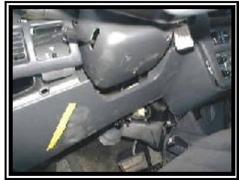
Figure 5. Scuff marks to the driver's knee bolster.
