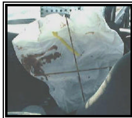
Figure 7. 1999 Chevrolet Cavalier Z24 deployed redesigned passenger air bag.
