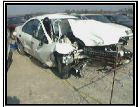
Figure 4. Front right damage to the 1999 Chevrolet Cavalier Z24.
