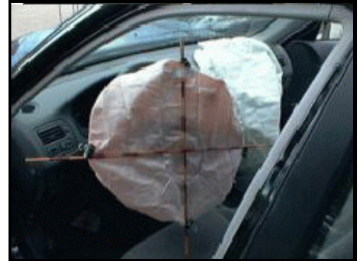
Figure 9. Deployed driver's air bag
