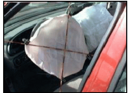
Figure 7. Deployed driver's air bag
