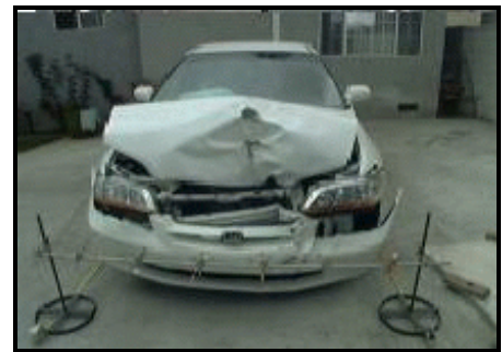
Figure 3. View showing frontal damage to Vehicle 2 (Honda)
