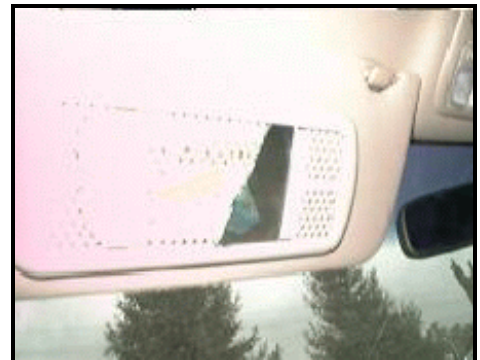
Figure 10. Damaged vanity mirror due to right hand contact
