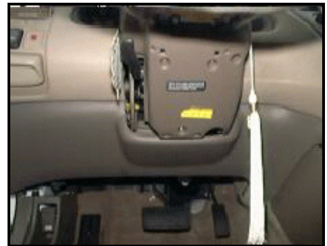
Figure 9. Close up showing knee contact to lower steering column cover
