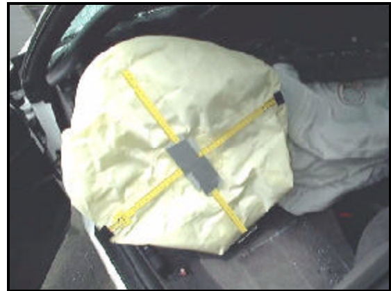
Figure 6. Driver's frontal redesigned air bag.
