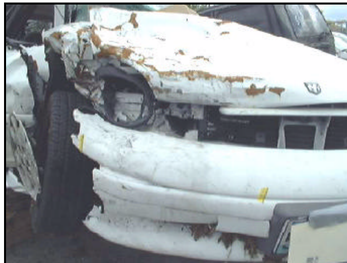
Figure 5. Direct damage, Vehicle 2 (1998 Dodge Neon 4-door)
