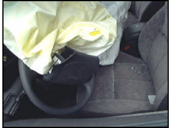
Figure 7. Driver's frontal air bag contact evidence.
