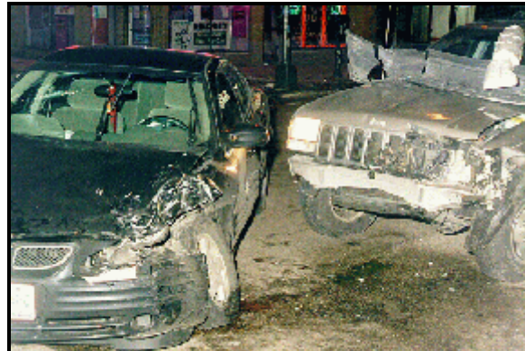
Figure 8: On-scene northeastward view of case vehicle (at left) and vehicle #2 (at right) at final rest; Note: initial contact involved vehicle #2's front left and the case vehicle's left front with a subsequent end slap between the front right half of vehicle #2 and the left front half of the case vehicle (case photo #12)
