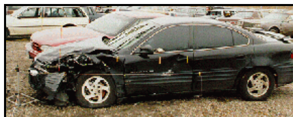
Figure 9: Case vehicle's left side damage extending from left front bumper to just past left "B"-pillar (case photo #18)
