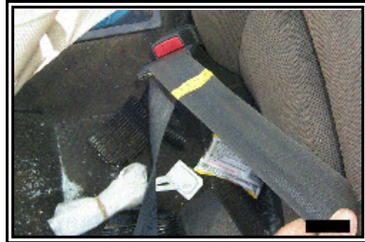
Figure 7- View of the small disruption of the lap belt webbing
