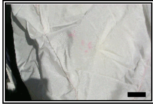
Figure 11- Close-up view of the red lipstick transfers on the inboard lateral surface of the front right passenger air bag
