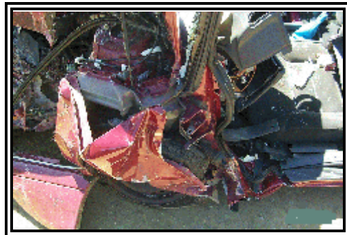
Figure 6- View of the left lower A-pillar and left sill showing the area cut and spread by rescue
