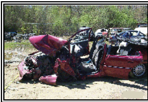
Figure 2- Damage resulting from the impact with the guardrail end
