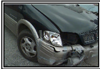
Figure 3. Front right damage to the Trans Sport.
