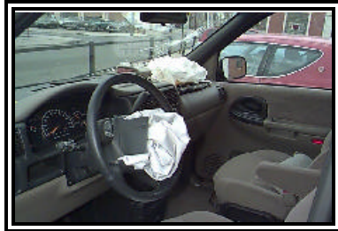
Figure 5. Overall view of the deployed frontal air bag system.
