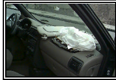
Figure 6. Top mounted front right passenger air bag module.
