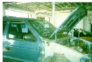
Figure 6- View of the damaged windshield glazing from contact with the expanding front right air bag
