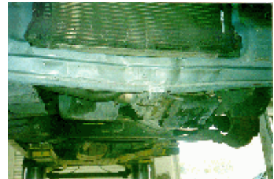
Figure 5- Close-up view of the contact damage to lower radiator support and center engine mount bracket
