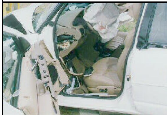
Figure 4: Case vehicle driver's seating area; Note, floor pan intrusion and displaced steering column (case photo #16)
