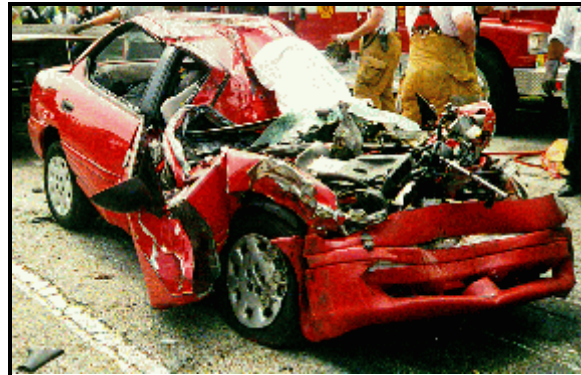
Figure 5: Case vehicle's frontal damage as viewed from the front right corner; Note: direct contact to roof rearward of the B-pillar (case photo #15)
