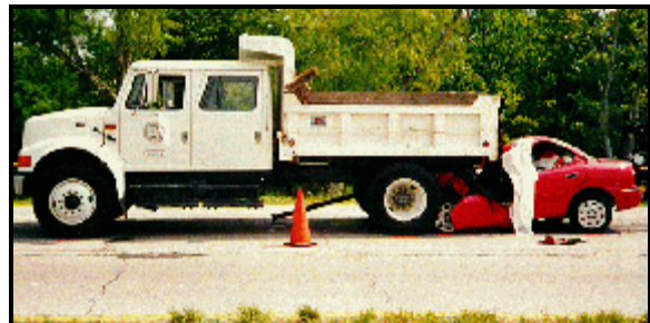
Figure 4: Final rest positions of the case vehicle and vehicle #2; Note: depth of underride by the case vehicle (case photo #05)
