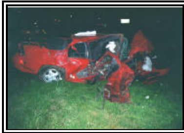
Figure 6. Right side damage to Chevrolet Monte Carlo
